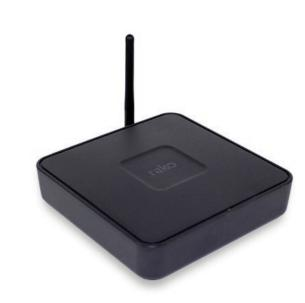
The Q-Hub is a programmable Rako to QMotion FM interface for QMotion motors only.
