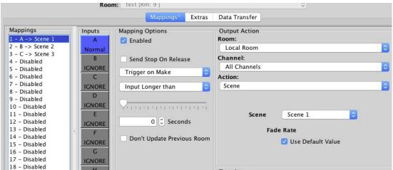
Above is an example of how a three way momentary switch would be programmed when wired into inputs A, B, and C of a WCM-D.
