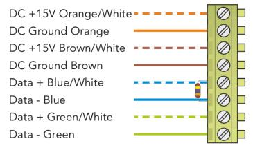
When the WCM-D is in the end of line position and not connected to a RAK-STAR a 120 Ohm resistor termination is required. This is provided with the WCM-D. The resistor is placed between the Blue and the Blue/White inputs.
