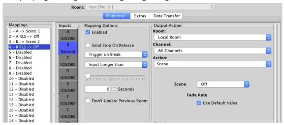
Above is an example of how a two-way latching switch would be programmed when wired into inputs A and B of a WCM-D.
