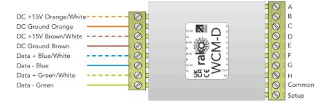
The WCM-D is wired into two pluggable sets of terminals. The 8-way terminal block connects to the Rako wired network formed of Cat5/Cat6 cable with cable allocations as set out above. The ten-way terminal block is used to wire between one and eight 3rd party
