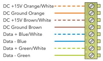
Used when the WCM-D is not at the end of line (with or without a RAK-STAR). This is usually identifiable by two cables being connected to the WCM-D.
