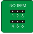
STAR TERM: Jumper fitted across 2+3 and 5+6 When a device is at the end of line, in a RAK-STAR System it must be STAR terminated.
