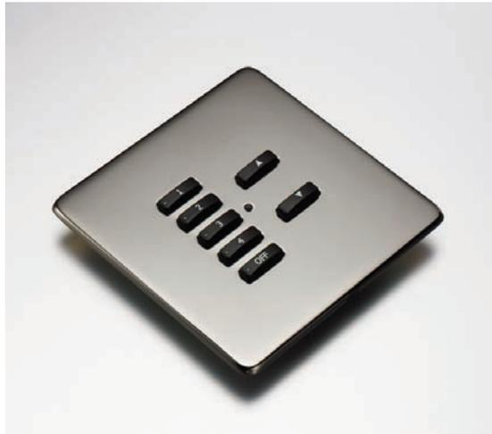
The RNC070 push button control module is programmable via Rako's patented NFC (Near Field Communication) technology allowing each of the buttons to trigger a single or multiple commands. Each input is fully customisable, can be addressed to separate Rako Rooms or Channels and activate on press, or release which gives a 'Press and Hold' function. Additionally each input can trigger an internal macro function.
