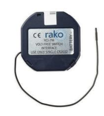
The RCI-7M accepts volt-free latching switch inputs and transmits wireless Rako wireless signals to other Rako wireless receiver and Hub units.
