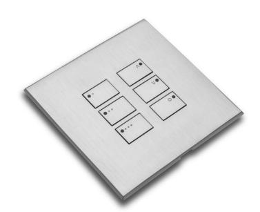
The WK-EOS push button wired control module is programmable via Rako's Rasoft Pro software. Each input is fully customisable and can be addressed to separate Rako Rooms or Channels and activate on press or release, giving a 'Press and Hold' function. Each button is complete with a blue LED indicator, additionally, each input can trigger an internal macro function.
